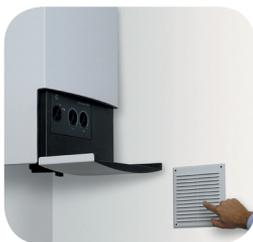
Stoves, water heaters and heating systems using the air in the house, referred to as types A and B, require a ventilation opening to ensure that the air they need for combustion is always available in the room in which they are installed. If this is not the case, they will slowly consume all the oxygen in the room, creating a danger for people and animals. And gas combustion will be incomplete, generating dangerous carbon dioxide. We might call this permanent opening a “safety entry”!
